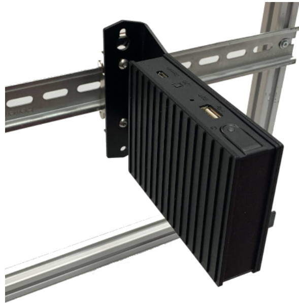
Figure 8: Device mounted on DIN top hat rail
