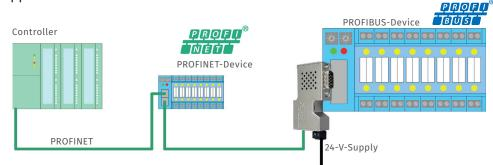
netLINK PROXY is plugged directly onto the PROFIBUS-DP connector of the slave. It is powered by 24 V. The RJ45 PROFINET jack is to be connected to PROFINET. The PROXY is configured via a PC with the configuration tool suite SYCON.net.
