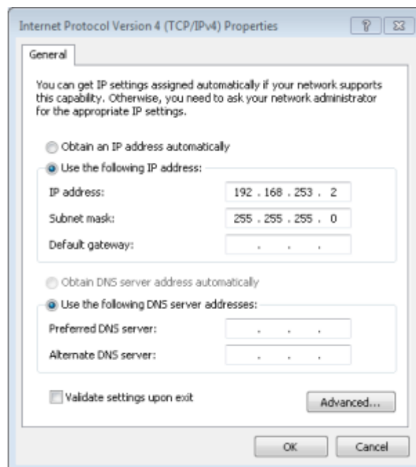
Figure 15: Setting IP address under Windows for direct LAN connection
