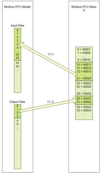
Figure 153: Examples - Reading Command with FC 3, Writing Command with FC16
