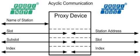
Figure 158: PROFINET – PROFIBUS Address Mapping
