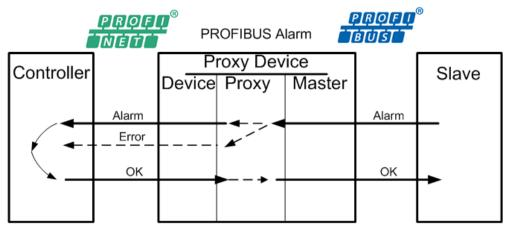
Figure 160: PROFINET IO- PROFIBUS DP – Alarm Errors
