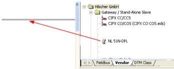
Or go to the device catalog under fieldbus **PROFINET IO** to the category **Gateway / Stand-Alone Slave**. Use drag and drop with the NL 51N-DPL proxy device to insert it at the (gray) main line.
