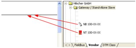
Figure 21: Insert Gateway Device into the Project
