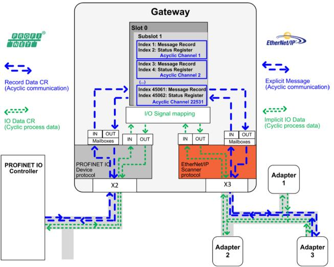
Figure 164: Acyclic Communication PROFINET IO-Device to Ethernet/IP Scanner
