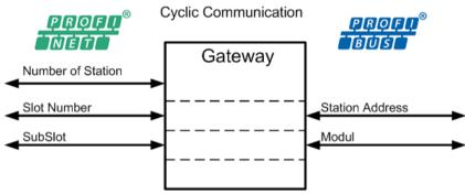
Figure 150: PROFINET – PROFIBUS Adress Mapping
