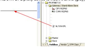
Figure 77: Insert Proxy Device into the Project
