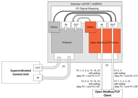
Figure 122: Access of the Open Modbus/TCP Client to the netTAP and netBRICK Device
