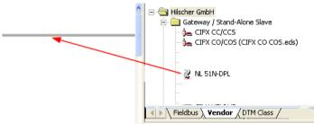
Or go to the device catalog under fieldbus **PROFINET IO** to the category **Gateway / Stand-Alone Slave**. Use drag and drop with the NL 51N-DPL proxy device to insert it at the (gray) main line.
