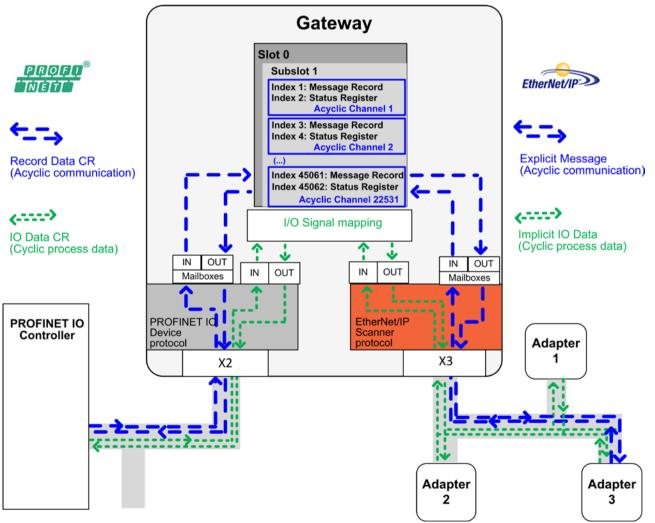
Figure 137: Acyclic Communication PROFINET IO-Device to Ethernet/IP Scanner
