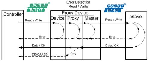
Figure 132: PROFINET IO – PROFIBUS DP Read/Write Error Detection
