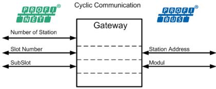
Figure 123: PROFINET – PROFIBUS Adress Mapping
