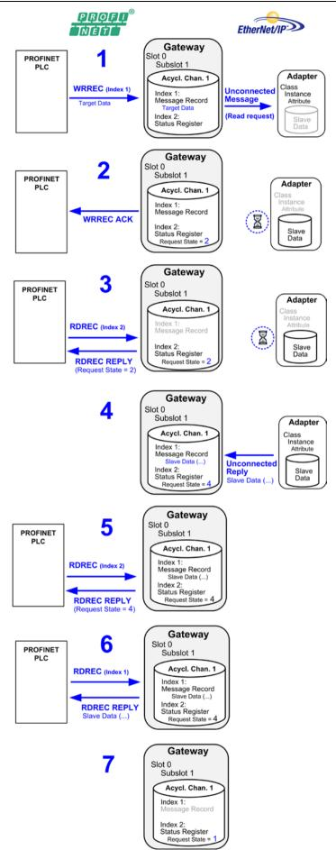
Figure 138: Sequence Acyclic Reading Task PROFINET to EtherNet/IP
