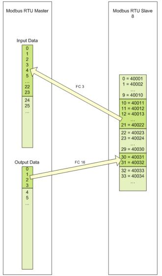
Figure 126: Examples - Reading Command with FC 3, Writing Command with FC16
