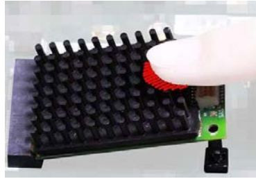
Figure 52: Press down the basic card with light pressure (max. 2 N) (example)
