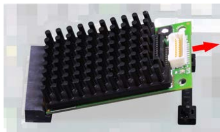
Figure 62: Remove PC card cifX from Mini PCI system connector
