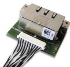
Figure 57: Connecting the Detached Network Interface Ethernet (AIFX-RE) to the Basic Card CIFX 104C-RE\F (Example)
