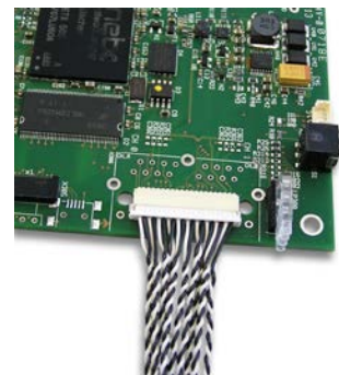
Figure 57: Connecting the Detached Network Interface Ethernet (AIFX-RE) to the Basic Card CIFX 104C-RE\F (Example)
