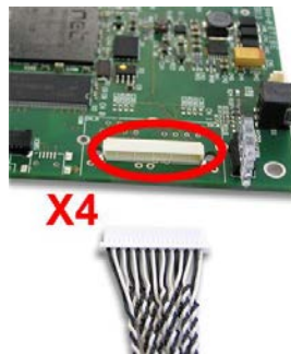
Figure 57: Connecting the Detached Network Interface Ethernet (AIFX-RE) to the Basic Card CIFX 104C-RE\F (Example)
